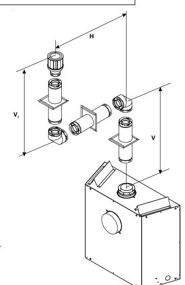
NOTE: There <u>MUST</u> be a 25% reduction in total H when using flex vent except when using the simple up and out installation (see Figure 9).
